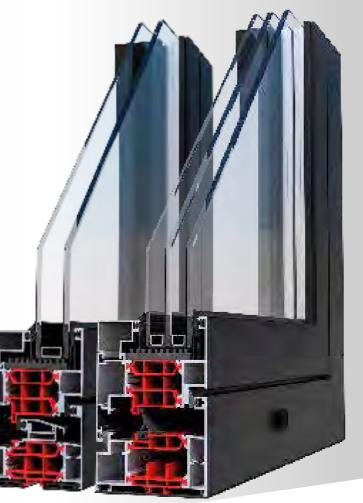
Albio 129C Advanced is the only system having a sash with a width of 78,3mm that presents high thermal-insulation properties with Uf=1,48 W/( $m^2$ K) and Uw=1,4 W/( $m^2$ K) Ug=1,0 W/( $m^2$ K), thanks to the use of special polyamides. The design of the system with minimal straight lines offers a minimalistic look and improved aesthetics. Furthermore, there is the possibility to use a frame that is coplanar not only at the outside but in the inside too.
